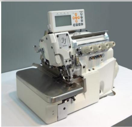
2 needles, 4 thread high speed overlock machine with automatic tape cutter with three sensors and air saving and the lint collecting device.
