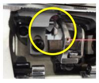
Adapted fixed type needle guard. Stitch length & differential ratio can be changed without adjusting the needle guard position.
