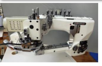
4 needles, 6 threads feed-off-the-arm, flatseamer for medium to thick fabric equipped with both side cut presser foot, direct drive servo motor, digital hand pulley, pneumatic suction device & foot lifter.
