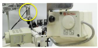
Direct drive servo motor, presser foot lifter & digital hand pulley are included.
