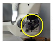
Stitch length & differential ratio can be adjusted by levers from out side of the machine.
