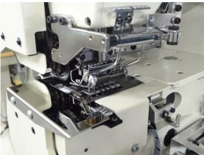
Needle feed mechanism ensures the strong and accurate feeding for heavy material
