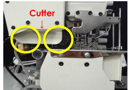
Double puller mechanism makes possible to cut materials properly by holding fabric with the front and rear puller.
