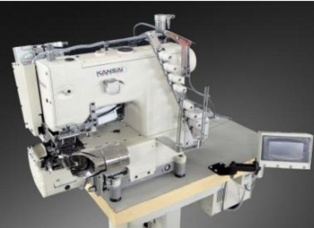
4 needle cylinder bed, double chain stitch machine for denim waistband attaching. The machine is equipped with edge sensor, fabric cutter, skip stitch device and digital puller system
