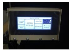
Operator friendly LCD touch screen Automatic mode on/off with a touch Easy to adjust the cutting length and skipping length.
