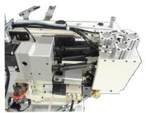
Rear puller, controlled by pulse motor makes possible various rear feeding pattern depending on material.
