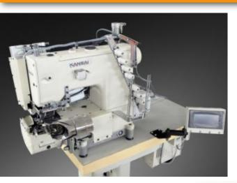
4 needle cylinder bed, double chain stitch machine for denim waistband attaching. The machine is equipped with edge sensor, fabric cutter, skip stitch device and digital puller system
