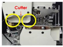
Double puller mechanism makes possible to cut materials properly by holding fabric with the front and rear puller.
