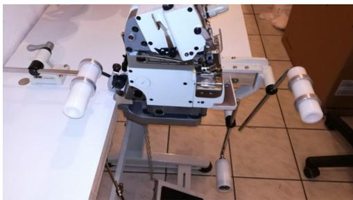
Attaching a roller set for expanding an elastic tape according to the diameter of the garment makes sewing very easy without any ply shifting
