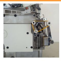
**Elastic insertion** It is suitable for over edge of the work glove wrist and inserting an elastic into it.
