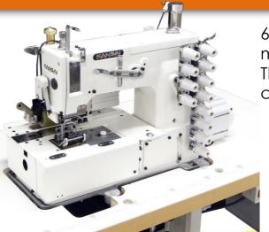
6 needle flat bed, double chain stitch machine for denim waistband attaching. The machine equipped with a fabric cutter, skip stitch device and foot lifter
