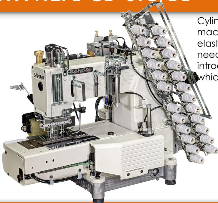
Cylinder bed, Multi-needle, double chain stitch machine with thread cutting device and elastic expanding device, Maximum 12 needles can be used. To prevent fraying, we introduce our condensed stitch mechanism which can be operated by lever.
