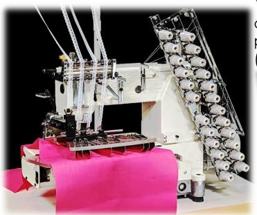
12 needle, cylinder bed, double chain stitch machine for pin-tucking with special folder.
