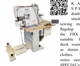
KANSAI SPECIAL's double chain stitch, feed sewing machine, the flagship model ofFBX series, is suitable for sewing thick waistbands such denim and work The clothes. **WFB** KANSAI series uses
