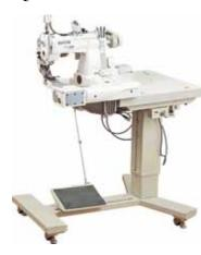
The "-DG" model, which will also be exhibited at the exhibition, is quipped with a patented independent needle guard mechanism in Japan. Which is three needle square type of feed-off-the-arm, double chain stitch machine.
