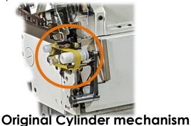
Cylinder mechanism suitable for rubberized working gloves
