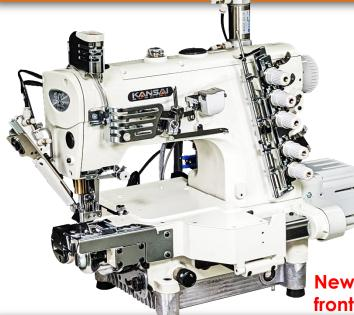
3 needle, small cylinder bed, top and bottom cover-stitch machine with a fabric trimmer built in the left side of needles and thread trimmer.
