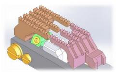
Differential feed mechanism ensures prevents puckering.
