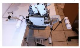
Attaching a roller set for expanding an elastic tape according to the diameter of the garment makes sewing very easy without any ply shifting
