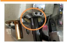
**Needle bar oil return system**Protects the fabric from the oil stain
