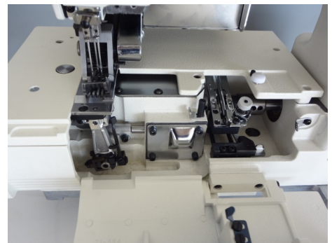
Micro adjustable looper holder Sliding style looper thread
