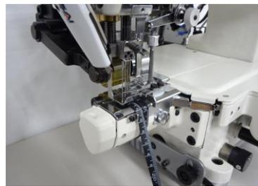
Equipped with an exterior looper thread take-up cam, it is easy to thread and adjust. The automatic thread trimmer increases productivity.
