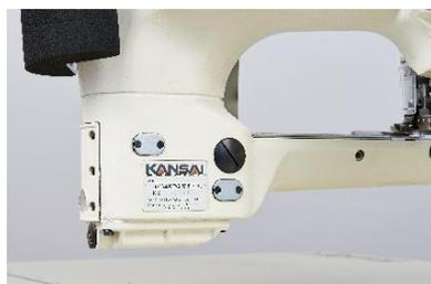
Differential feeding mechanism was developed with a wider range of differential ratio. It can be adjusted from 1 : 1.5 to 1 : 0.5 by switching the position of the feed rocker.
