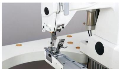
This model is equipped with a guillotine tape cutter operated by push button. A tape folder (finish size 10 mm) is included in the machine.
