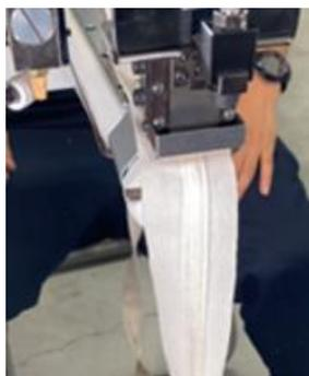
This model is equipped differential feed dog mechanism. By adjusting the differential ratio of front & back feed dog, puckering can be eliminated.
