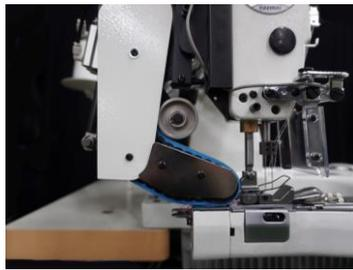
Newly developed original puller system realizes more powerful fabric feeding. Seam portion on the materials can cross stably and beautifully. The feed amount can also be adjusted easily.
